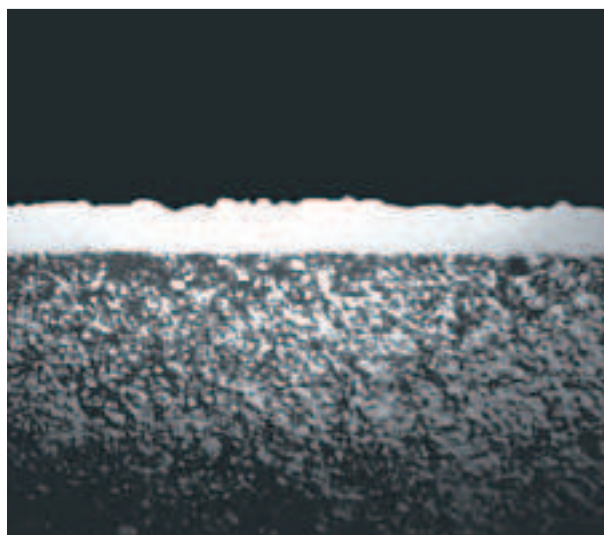
Fig. 8.2: Cross section of the ATCoat coating
