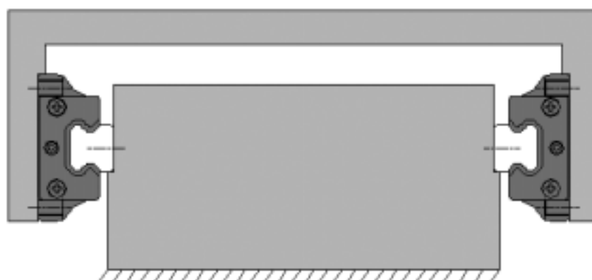
(C) Su piano verticale con pattini traslanti (C) Vertical plane with free blocks
